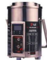
SMA MicroPortable 28.3/141.5 L/min, 25 mL agar D_{50} = 4.8 \mu\text{m}
