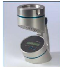
MAS-100 100 L/min, 50 mL agar D_{50} = 1.7 \mu\text{m}
