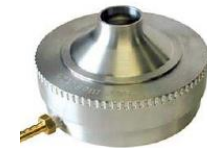
BioStage 28.3 L/min, 50 mL agar D_{50} = 0.65 \mu\text{m}
