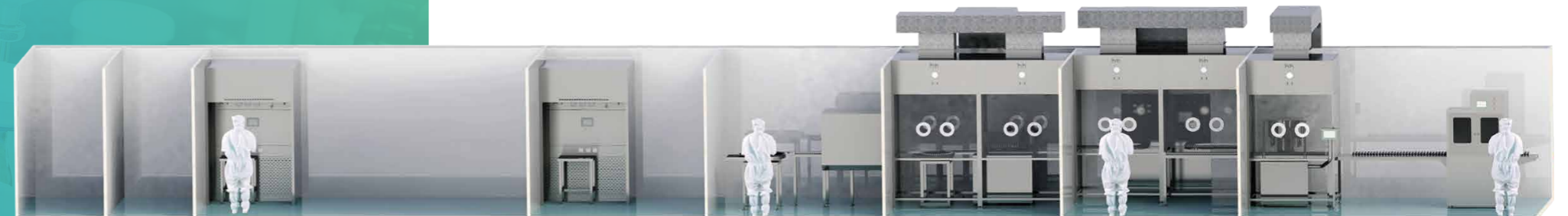
Changing Air Lock Raw material weighing Active carbon weighing Washing drying bottle Encapsulation Lyophilization Capping Light inspection
